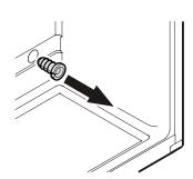
Pull out strain relief device.
