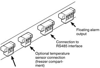
Optional temperature sensor connection (refrigerator compartment)
